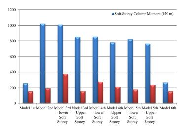
**Graph 4** Bending Moments of Different Models of Building Frame in Longitudinal Direction
