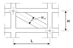
Fig.6 Compression diagonal model
