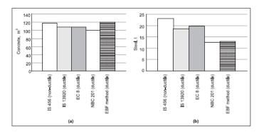
Fig.7 Quantity of concrete and steel in building with various building code procedures.
