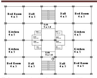
Fig.9. Proposed Line Plan of RCC Apartment Building
