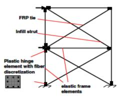
Fig.8 Analytical structural model
