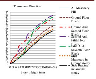
**Graph 1** Lateral Deflection of Different Models of Building Frame in Transverse Direction
